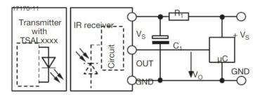
$R_{\rm 1}$  and  $C_{\rm 1}$  recommended to reduce supply ripple for  $V_{\rm S}$  < 2.8 V
